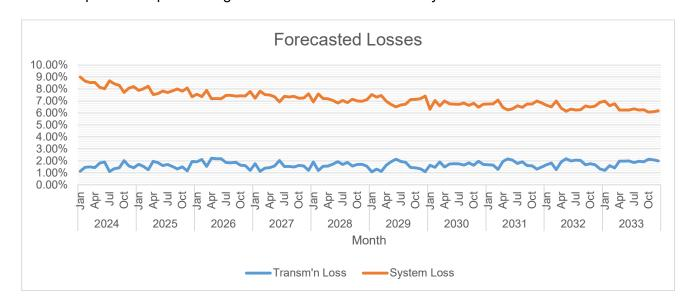
Transmission Loss varies from 1.15% and 2.22%. The Total System Loss (Sub-transmission, Substation, and feeder loss) is expected to decrease from 9.01% January 2024 to 6.06% by the end of 2033.
